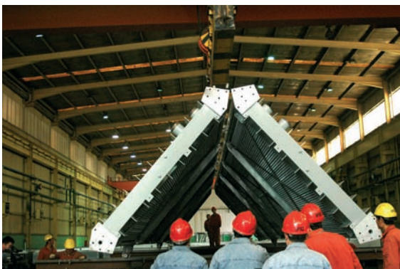
Tube bundles assembled into a Delta shape
