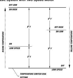
Sequence of Operation Basic System with Two Speed Motor
