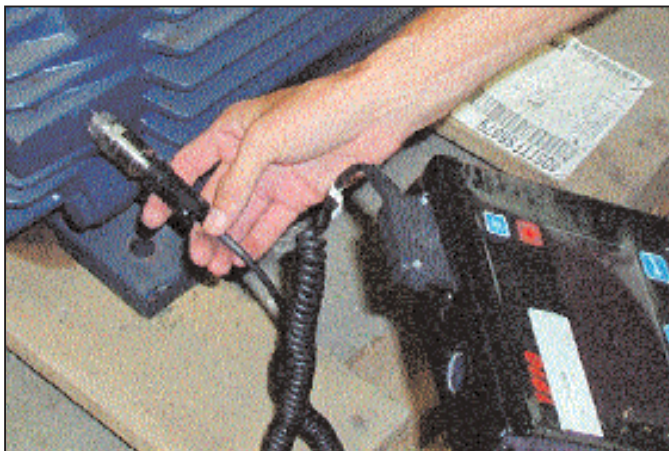
Use a handheld vibration analyzer to check mechanical operations.
