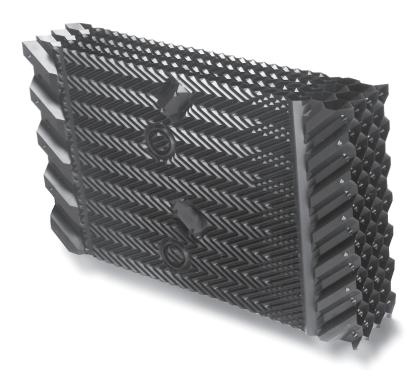
The single most important component of a cooling tower is the fill. The efficiency of a cooling tower depends upon the fill's ability to promote both the maximum contact surface, and the maximum contact time between air and water. And it must promote this air-water contact while imposing the least possible restriction to air flow.
