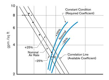
FIGURE 8 Cooling tower characteristic, KaV /L versus gpm /sq ft. Correlation lines and plotted points identical to those in Figure 7.
