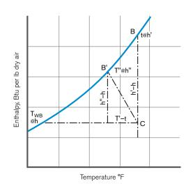
FIGURE 9 True versus apparent potential difference
