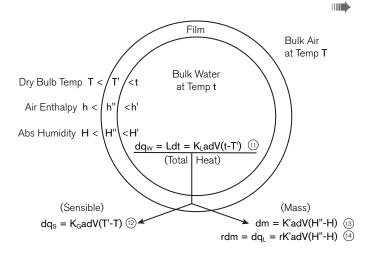
FIGURE 1 Heat and mass-transfer relationships between water, interfacial film and air. Numbers in circles refer to equations in Appendix A.
