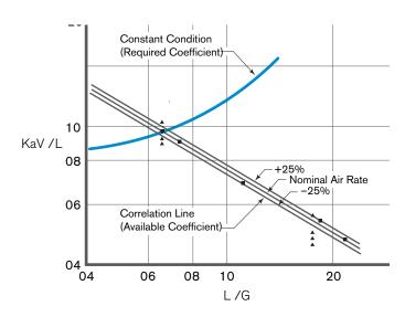
FIGURE 7 Cooling tower characteristic, KaV /L versus L /G. Platted points at nominal air rate. Square points at 100° hot-water temperature. Triangular points vary from 80° to 160° hot-water temperature.
