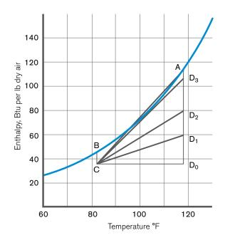
FIGURE 6 Counterflow cooling diagrams for constant conditions, variable L/G rates
