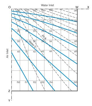
FIGURE 3 Water temperature and air enthalpy variation through a crossflow cooling tower
