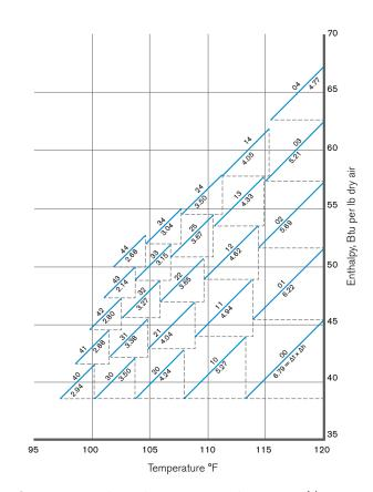
FIGURE 5 Plot of crossflow calculations from Table 1(c)
