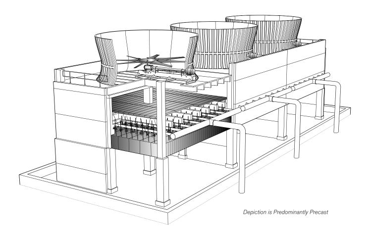
**800 class** cooling towers are mechanical draft, film fill, concrete counterflow cooling towers. Although designed to serve all cooling water systems, the construction described in this specification applies primarily to the rigors associated with seawater service.
