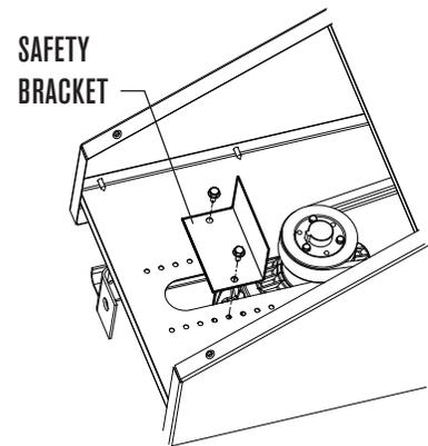
On 8.5' wide models, the fan motor and belt adjustment mechanism is located outside the fluid cooler. Remove the motor protection hood by loosening the two thumbscrews on top and hinge the hood up and out of the way. Also, remove the motor sheave safety bracket and set aside. See the following images. On 10' and 12' wide models, the motor is located inside the fluid cooler plenum. Open the access door (see Access Door Operation) and hinge out of the way.
