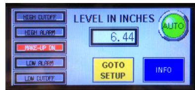
3. Enter the setup sequence by pressing GOTO SETUP.
