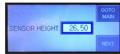
6. Press next to enter the water level programming screens. Enter water level setpoints by pressing the light blue cell and entering a value on the yellow keypad. Then press ENT to save the entry.
