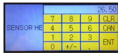
5. When prompted enter the measured sensor height distance.
