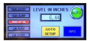
Boxes highlighted in red indicate the relay inside the control panel has been energized.
