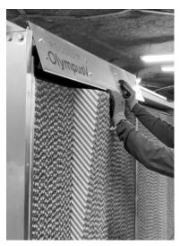
3 With top of pad free from basin, lift the pad out of the lower tray.
