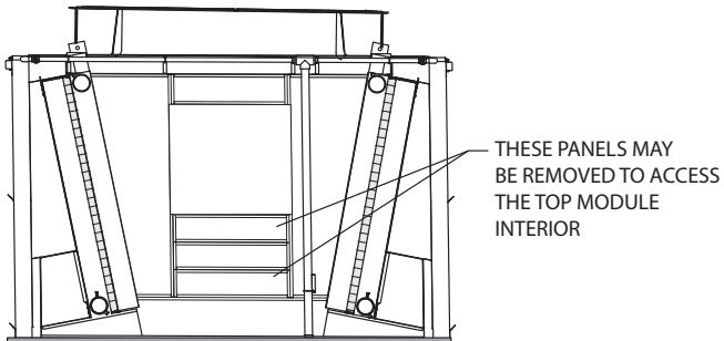
Panels are assembled with sixteen (16) M8 bolts around the perimeter of each panel that will have to be removed. Use 13mm or  $\frac{1}{2}$ " sockets and wrenches for removal. To reinstall, use the turn-of-the-nut method with a  $\frac{1}{4}$  turn past snug tight. Fasteners may be reused provided they're not damaged.
