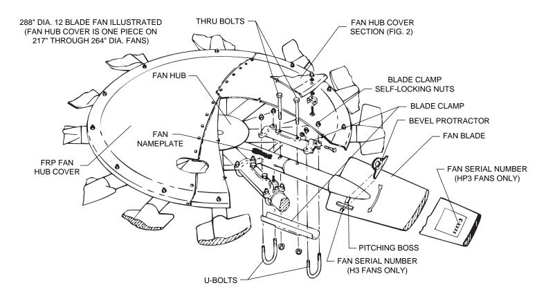
**Welded Hub Fan Assembly**
