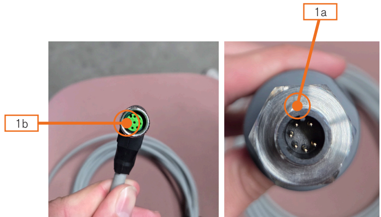
Figure 4: Probe and Sensor Cable Keyhole
