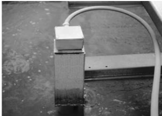
Stilling chamber used to support hanging probes or ultrasonic sensor
