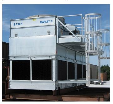
MARLEY MD COUNTERFLOW COOLING TOWER Counterflow, induced-draft design requires less plan area than crossflow towers. Factory assembly and G-235 galvanized steel construction are standard. Five-year mechanical equipment warranty. Tower capacity from 89 to 756 tons per cell. CTI and Eurovent Certified. FM Approved models available.
