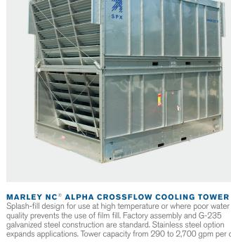
Splash-fill design for use at high temperature or where poor water quality prevents the use of film fill. Factory assembly and G-235 galvanized steel construction are standard. Stainless steel option expands applications. Tower capacity from 290 to 2,700 gpm per cell.
