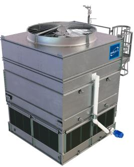
**MARLEY MC CLOSED-CIRCUIT COUNTERFLOW FLUID COOLER** Forced draft design with centrifugal fans allows quiet indoor operation. G-235 galvanized steel factory-assembled structure. Also available in 300 series stainless steel. The ideal solution for sound- and spacesensitive applications.
