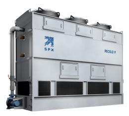
**RECOLD LC COUNTERFLOW EVAPORATIVE CONDENSER** Induced-draft design with copper coil and patent-pending heat-transfer technology. Reduces refrigerant charge up to 40 percent and lowers fan energy consumption up to 50 percent.
