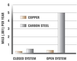
Adapted from *Standards for Corrosion Rates*, Bennett P. Boffardi, Ph.D., FNACE
