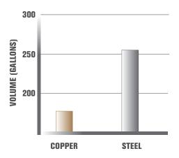
Internal coil volume typical of a 100 ton forced-draft fluid cooler
