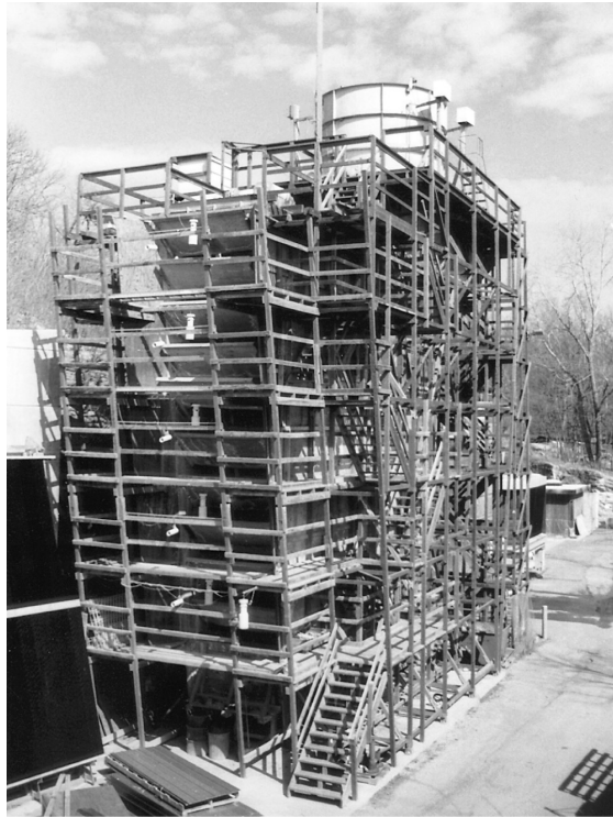
Five-story industrial size crossflow test cell
