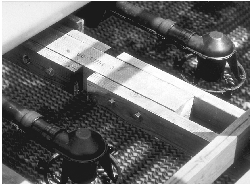
Figure 1—Marley splice joint
