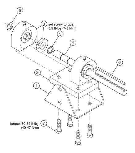
Installation: Installation should only be performed by a qualified technician. Lockout and disable any system drivers. Coat the shaft(s) with a lubricant or anti-seize compound. Follow the instructions supplied with your replacement kit or the tower manual. Contact Marley should you need more information for your application.
