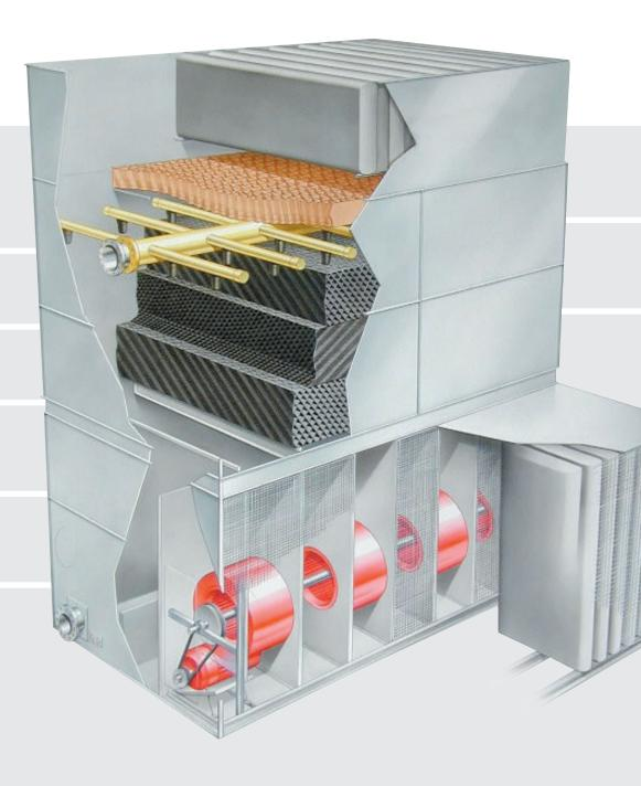
The Marley MCW maximizes forced-draft, counterflow technology and high-performance fill media to deliver fully-rated cooling over a wide range of flow and temperature requirements.
