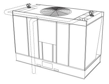
If each cell is to be equipped with an outlet, cased-face outlets can be used on end cells of multicell towers, but a cased-face outlet cannot be used on interior cells. For direct outlet from each cell on installations of three or more cells, use either the depressed sump or bottom outlet on interior cells.
