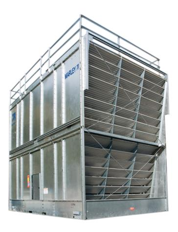
**NC Alpha** towers are steel structure, splash fill, factory assembled, crossflow cooling towers, designed to serve all normal cooling water systems—as well those "dirty water" systems which would place the long term operation of a film fill tower in jeopardy. They evolve from a factory-assembled concept of towers pioneered by Marley some 60 years ago, and incorporate all of the design advancements that our customers have found valuable.
