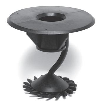
The Marley NX 250 is a crossflow cooling tower nozzle with an extra-large, clog-free orifice. The NX 250 nozzle has several orifice diameters up to  $2\frac{1}{2}$ ". With its smooth self-cleaning water deflector bottom ring, the NX 250 exhibits the same distribution characteristics as smaller, closer spaced nozzles. NX 250 nozzles are normally spaced on  $2^{\prime}$ - $0^{\prime\prime}$  centers.
