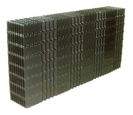
Marley AAFNCS™ anti-fouling film fill consists of thermoformed corrugated sheets made of rigid polyvinyl chloride (PVC), impervious to decay, fungus and biological attack. The sheets are bonded to form modules which can be dimensioned to fit any application.
