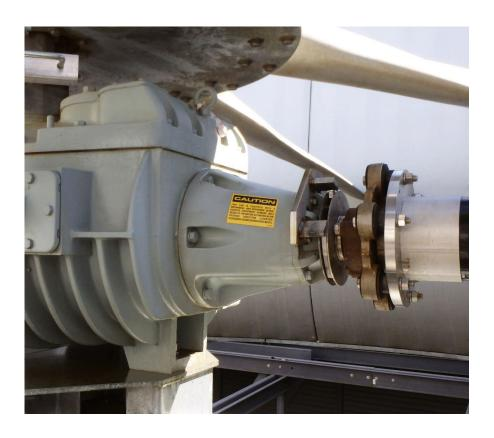
The Marley external Disc Anti-Reversing Device (ARD) backstop is a custom designed, welded stainless steel assembly that is bolted directly to a Marley Geareducer® with input shaft diameters from 1.125" up to 2.625". Specifically designed for all right-angle Geareducer models the Disc ARD prevents reverse rotation of the fan, Geareducer and motor and can be field installed.
