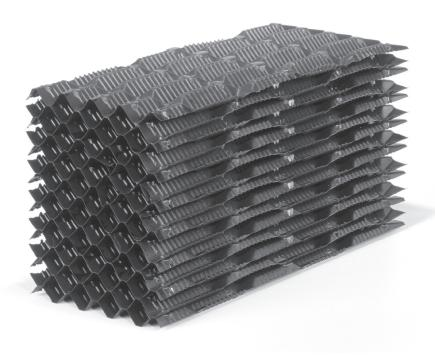
Marley FB20 clog-resistant film fill is constructed of fire-retardant PVC sheets bonded to form blocks of cooling media. The surface microstructure facilitates air/water mixing and increases the surface cooling area. The offset vertical flutes provide directional changes in air and water flow to increase cooling and promote thermal efficiency while substantially reducing the occurrence of fouling.
