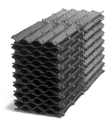
The Marley FC18 clog-resistant film fill is constructed of fire-retardant PVC sheets bonded to form blocks of cooling media. The microstructure on the surface of the sheets increases the cooling area and aids the cooling process. The vertical flutes allow even water flow through the media to minimize fill fouling.
