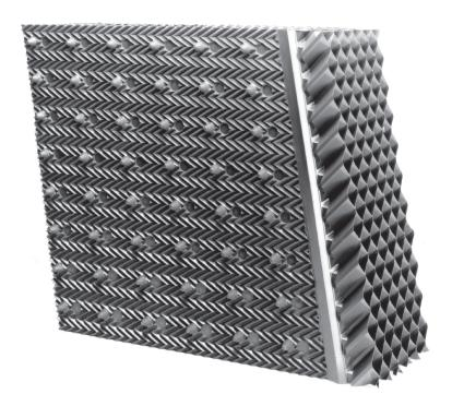
The fill section is the heart of any cooling tower. Sometimes called packing, filling, or baffles, this is the area where water and air mix to achieve the cooling effect. A cooling tower can only perform if the fill material is in good condition, providing the greatest possible heat transfer surface.
