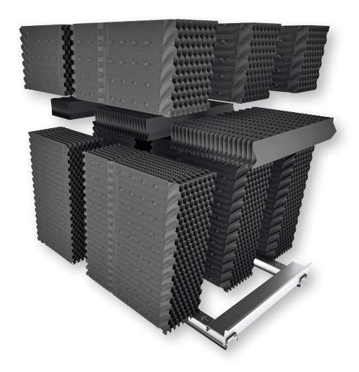
Marley MBX EZ Pack fill is a highperforming, bottom-supported, two-piece PVC pack fill with integral louvers and drift eliminators, specifically designed for fill replacement projects. The contractorfriendly fill design makes installation fast and easy without requiring major tower modifications.
