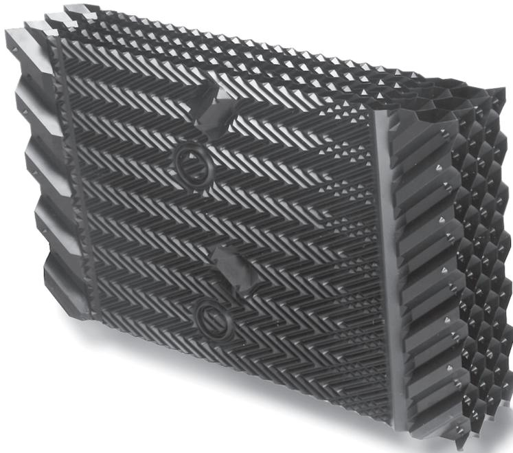
The single most important component of a cooling tower is the fill. The efficiency of a cooling tower depends upon the fill's ability to promote both the maximum contact surface, and the maximum contact time between air and water. And it must promote this air-water contact while imposing the least possible restriction to air flow.
