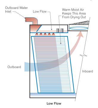
The inboard portion of the fill, however, is not dry. Since airflow in a crossflow cooling tower is horizontal across the flow of the falling water in the fill, there is still a tendency of the airflow to pull the water back into that section of the fill. Further, the air picked up moisture as a result of passing through the outboard section of fill and is now saturated.
