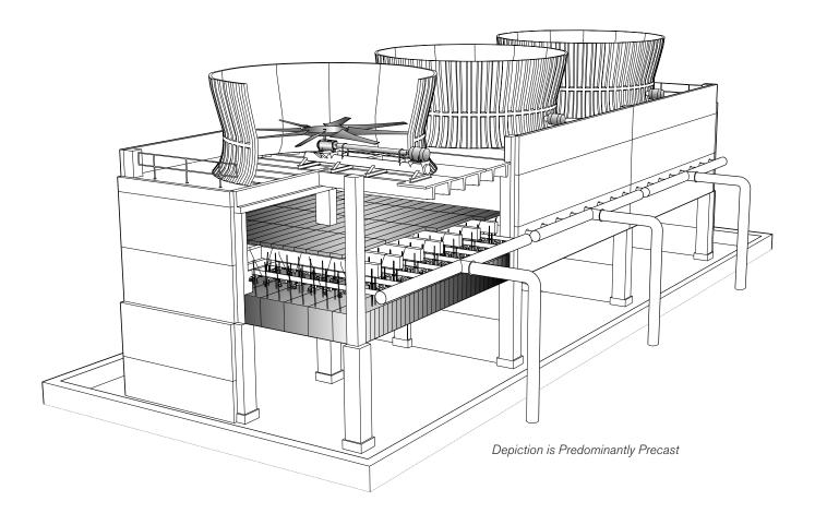
**800 class** cooling towers are film-fill, concrete counterflow cooling towers designed to serve all cooling water systems. They utilize both precast and formed-in-place construction techniques to meet the fast track schedules and competitive pricing required in today's market. The new 800 cooling tower incorporates the latest cooling tower technology—both in structure and components—developed in over 90 years of cooling tower experience.
