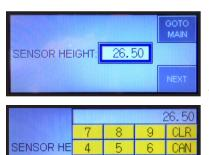
Press the light blue screen cell to right of SENSOR HEIGHT to bring up a yellow keypad then enter the sensor height in inches. Sensor height is from bottom of the sensor to basin floor (or bottom of PVC tubing in case of an external stilling chamber.
