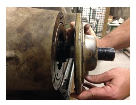
Figure 3. Slide the seal, pinion cap, and shims over the shaft until the cap bears against the pinion cage mating surface.
