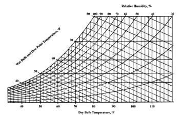
Relative humidity measures the difference between moisture actually in the air and the amount of moisture the air could hold. In evaporative cooling systems, heat is transferred based on wet bulb, while dry systems rely on dry bulb. When relative humidity is low, evaporative cooling becomes more beneficial.
