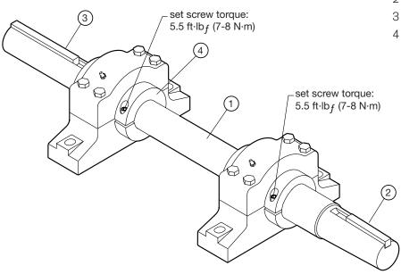
**Installation:** Installation should only be performed by a qualified technician. Lockout and disable any system drivers. Coat the shaft(s) with a lubricant or anti-seize compound. Follow the instructions supplied with your replacement kit or the tower User Manual. Contact your Marley sales representative should you need more information for your application.
