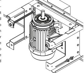
On 10' and 12' wide models, the fan motor is located inside the plenum of the fluid cooler. The motor can be accessed through the mechanical access panel. See the **Access Door Operation** section for instruction on opening the access panel. Remove the drive belt by following the instructions in the **Belt Tensioning** section.
