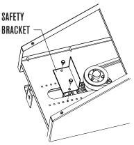
On 8.5' wide models, the fan motor and belt adjustment mechanism is located outside the fluid cooler. Remove the motor protection hood by loosening the two thumbscrews on top and hinge the hood up and out of the way. Also, remove the motor sheave safety bracket and set aside. See the following images.
