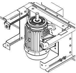
On 10' and 12' wide models, the fan motor is located inside the plenum of the fluid cooler. The motor can be accessed through the mechanical access panel. See the **Access Door Operation** section for instruction on opening the access panel. Remove the drive belt by following the instructions in the **Belt Tensioning** section.
