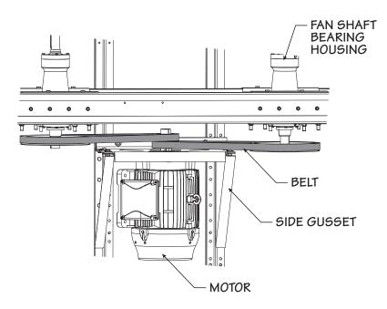
Figure 3 Single Motor-Two Fans
