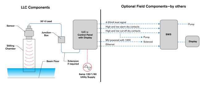
The Liquid Level Control systems are used to accomplish five different functions:
