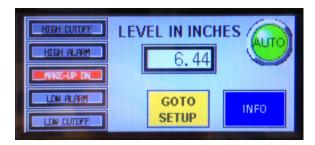
Red indicates the relay inside the control panel has been energized.
