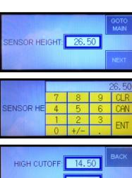
Press the light blue screen cell to right of SENSOR HEIGHT to bring up a yellow keypad then enter the sensor height in inches. Sensor height is from bottom of the sensor to basin floor (or bottom of PVC tubing in case of an external stilling chamber.
