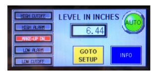
Red indicates the relay inside the control panel has been energized.
