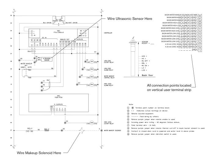
Wiring diagram is typical. Refer to wiring diagram on inside of the enclosure door for actual as-built wiring diagram, which may include project specific options.
