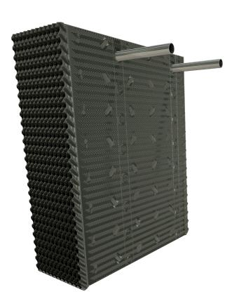
The single most important component of a cooling tower is the fill. The efficiency of a cooling tower depends upon the fill's ability to promote both the maximum contact surface, and the maximum contact time between air and water. And it must promote this air-water contact while imposing the least possible restriction to air flow.
