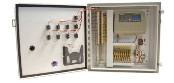
A main circuit breaker disconnect provides a true single point power connection for cooling tower controls. Contractor connects a single power source and the panel provides power feeds, controls and voltages for tower controls. Typically each cell of a tower requires one SPPC panel.
