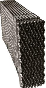
Drift rate varies with design water loading and air rate, as well as drift eliminator depth and number of directional changes. The exclusive patented MarKey' drift eliminators achieve the lowest available drift rates so less water escapes the tower. A drift rate of 0.0005% is readily available on many standard models. If a lower rate is required, please discuss with your Marley sales representative.
