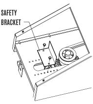
On 2.6m wide models, the fan motor and belt adjustment mechanism is located outside the fluid cooler. Remove the motor protection hood by loosening the two thumbscrews on top and hinge the hood up and out of the way. Also, remove the motor sheave safety bracket and set aside. See the following images. On 3 and 3.6m wide models, the motor is located inside the fluid cooler plenum. Open the access door (see Access Door Operation) and hinge out of the way.
