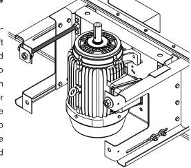
On 3 and 3.6m wide models, the fan motor is located inside the plenum of the fluid cooler. The motor can be accessed through the mechanical access panel. See the **Access Door Operation** section for instruction on opening the access panel. Remove the drive belt by following the instructions in the **Belt Tensioning** section.
