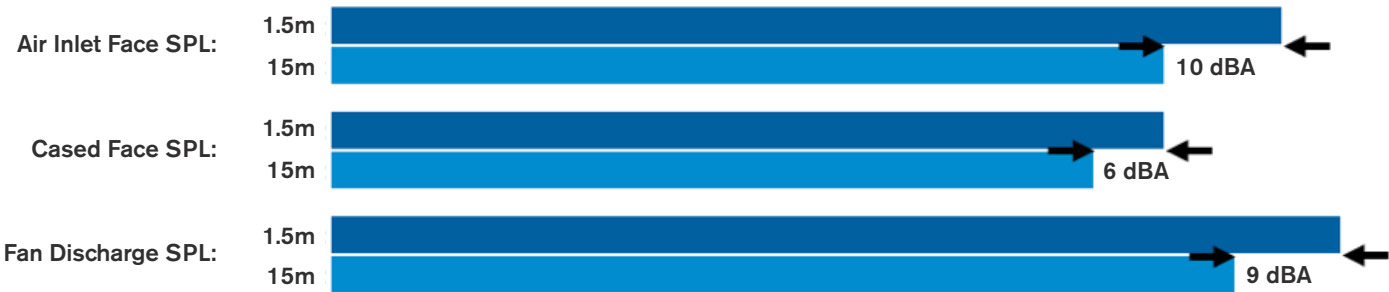
Figure 1: SOUND PRESSURE LEVELS (SPL) In Crossflow Induced-Draft Cooling Tower
