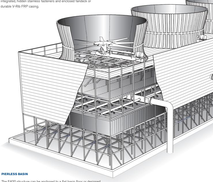
The F400 structure can be anchored to a flat basin floor or designed to fit existing basins. Fewer piers mean lower basin cost.
