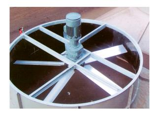
The mechanical equipment support needs to be designed and manufactured to maintain alignment of rotating parts.
