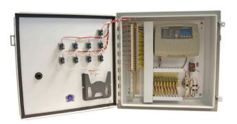
A main circuit breaker disconnect provides a true single point power connection for cooling tower controls. Contractor connects a single power source and the panel provides power feeds, controls and voltages for tower controls. Typically each cell of a tower requires one SPPC panel.
