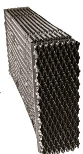
Drift rate varies with design water loading and air rate, as well as drift eliminator depth and number of directional changes. The exclusive patented MarKey\* drift eliminators achieve the lowest available drift rates so less water escapes the tower. A drift rate of 0.0005% is readily available on many standard models. If a lower rate is required, please discuss with your Marley sales representative.
