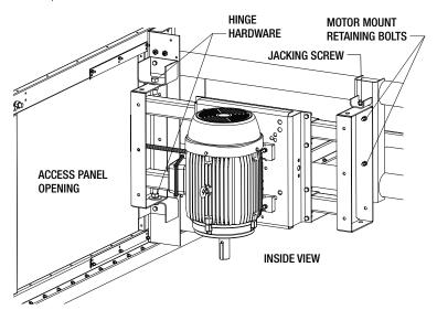
Hoisting attachment locations vary by motor - choose strap or chain attachment locations carefully to provide a balanced lift.
